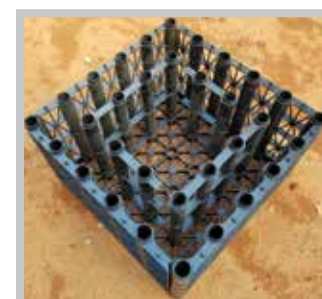
Fig. 11 For UD modules, two internal plates are removed, and two half-pieces are reinserted perpendicular to the other internal pieces.
