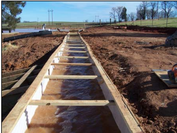
Figure 2. Gravity Flow to Flume
