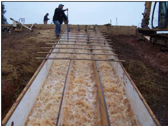
Figure 3. Channel Flow Velocity Measurement (typical)
