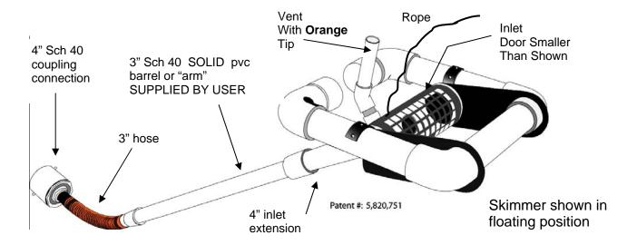
2. Glue the 8' long 3" sch 40 barrel to the 3" grey coupling on the hose.
