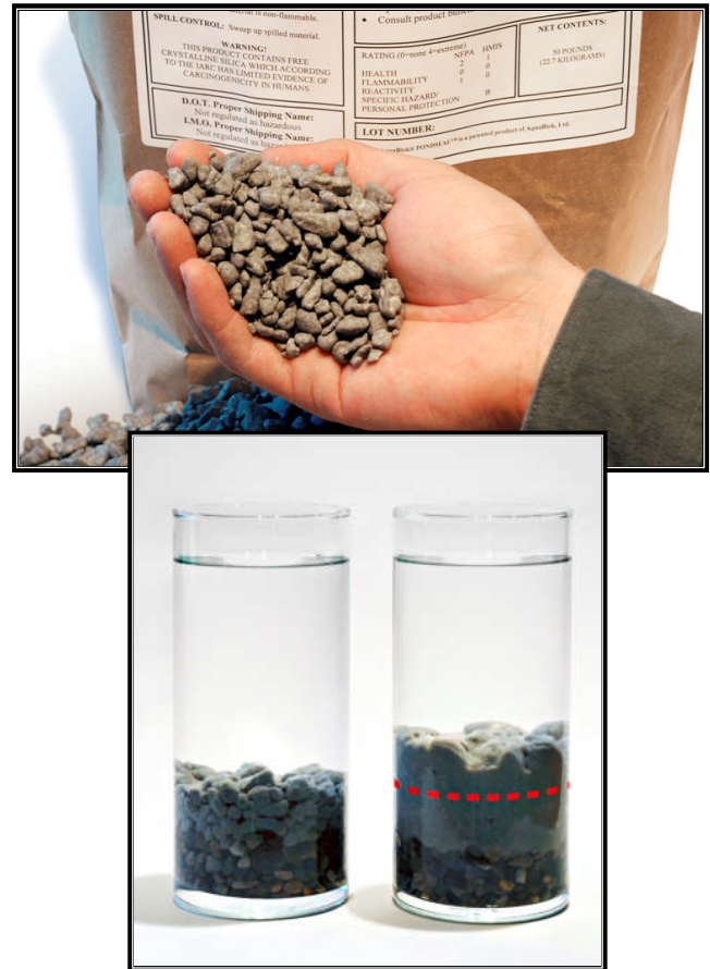
Figure 1. Configuration of stone-clay composite particle.
