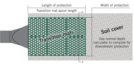
Culvert outlet protection – plan view
