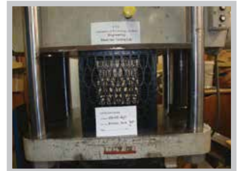
Unconfined Compression Test
