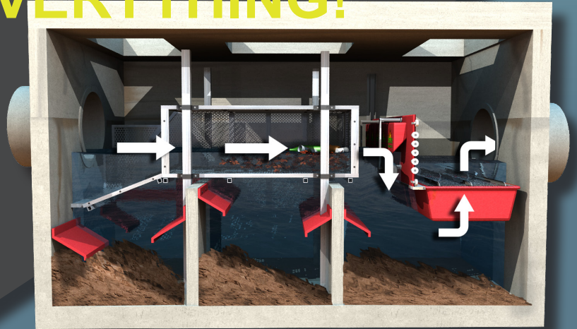
Bottom of concrete structure is only 4' below the pipe.
